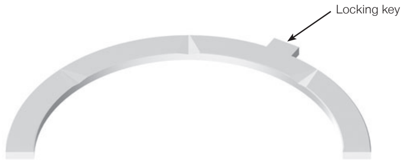
Figure 2. Axial thrust bearing with undamaged locking key
